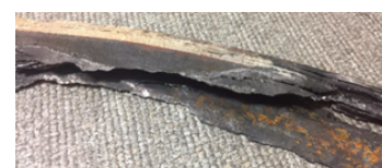
Difference in compression amount after installing eccentricity (top and bottom) Damage to Hiflex Gasket after use due to occurrence However, no leak with the performance of 3st O-Ring
